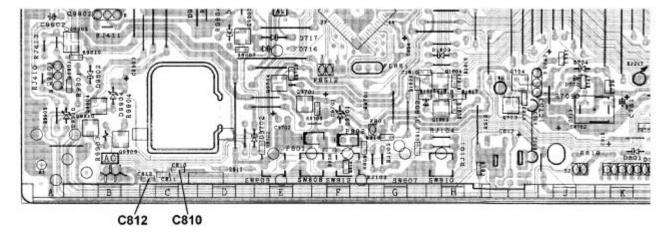
Note that C810 and C812 are located at the front edge of the Main PWB (left hand side as viewed from the front of the machine)
